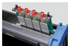
Plug-in slot for the input units
